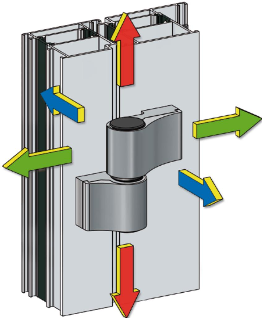
The Loira+ hinge in either two and three-leaf version, is adjustable in the three directions, when the door is in the closed position. Adjustments are micrometric and independent of one another.
