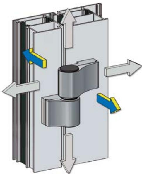
The micrometric adjustment in pressure of the gasket, of  $\pm 0,5$  mm, is carried out when the door is in the closed position, by rotating the lower bush and then locking the dowel.
