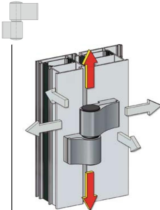
The micrometric vertical adjustment, from 0 to +4 mm, is carried out when the door is in the closed position through a stainless steel adjusting element, pre-assembled on the lower bush.
