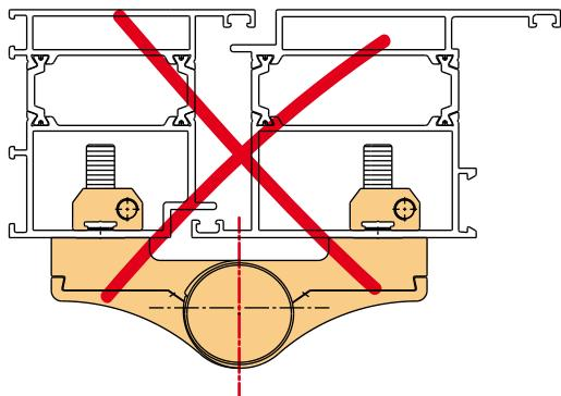
The special self-threading screws can be exclusively used on profiles having tightening catching on at least two profiles walls.
