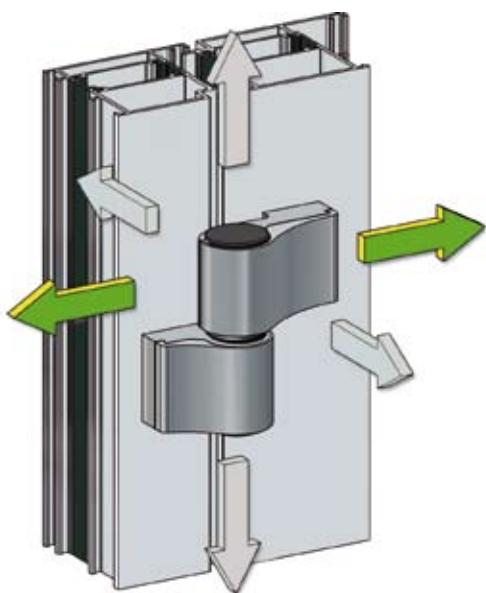
The micrometric horizontal adjustment, of  $\pm 2,5$  mm, is carried out when the door is in the closed position, by rotating the upper bush and then locking the dowel.
